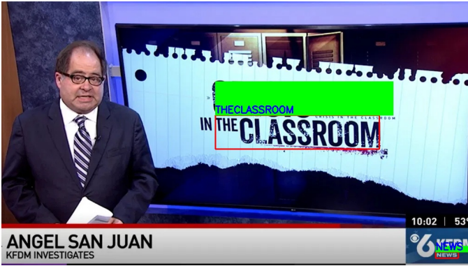
Fig. 2. Example of Aho-Corasick helping in identifying matches. Here the vocabulary contains the word “classroom”. However, the transcription detected is “THECLASSROOM”. In this case, Aho-Corasick is able to match the substring “classroom” to the vocabulary.
