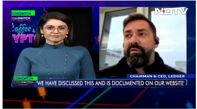
Fig. 3. Example of Levenshtein Distance helping in identifying a match. Here the vocabulary contains the word “coinswatch”. However, the text appearing in the frame is “coinswitch”. Levenshtein Distance between the two is 1 and so, “coinswitch” is flagged
