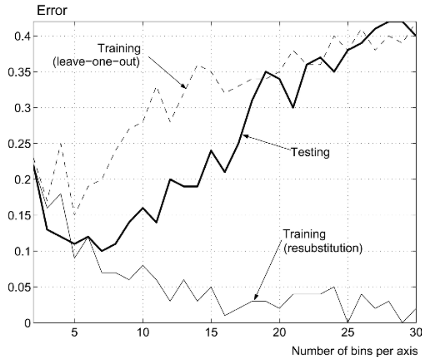
Fig. 2.3 Resubstitution, leave-one-out and testing error rates of the histogram classifier versus the number of bins per axis.
